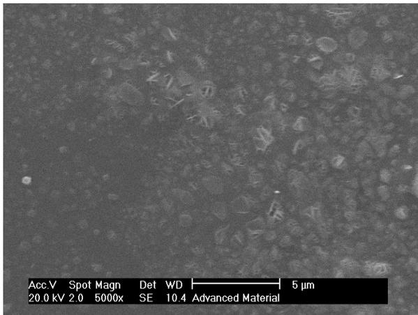
**Figure 2: Scanning electron microscopy of Al doped ZnO (0.9 concentration) thin film by CBD method**
