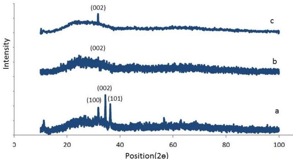
**Figure 4: XRD pattern of AZO thin layers produced by CBD method, a) ZnO layers, b) Al doped ZnO(0.9 concentration), c) Al doped ZnO (1 concentration)**
