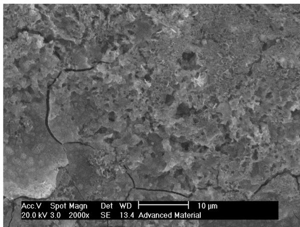
**Figure 3: Scanning electron microscopy of Al doped ZnO (1 concentration) thin film by CBD method**
