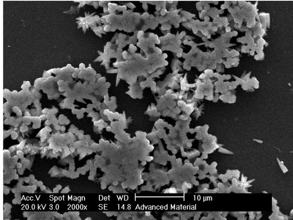
**Figure 1: Scanning electron microscopy of ZnO/glass thin film by CBD method**
