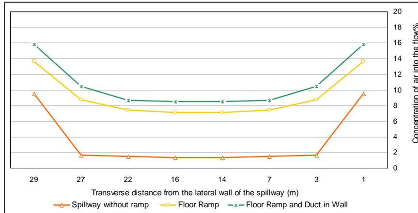
**Figure 8: Changes in the concentration of air into the flow in cross section at a distance of 260 meters from the zero**
