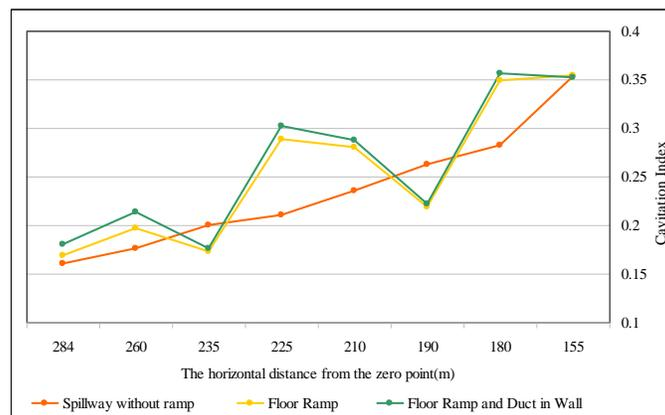
**Figure 3: Changes in the cavitation index in 3 spillway models in discharge of 2290 m<sup>3</sup>/s**
