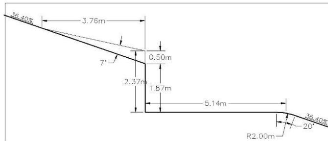
**Figure 2: Size and shape of the ramp modeled in the spillway**
