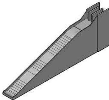
**Figure 1: The primary spillway**
