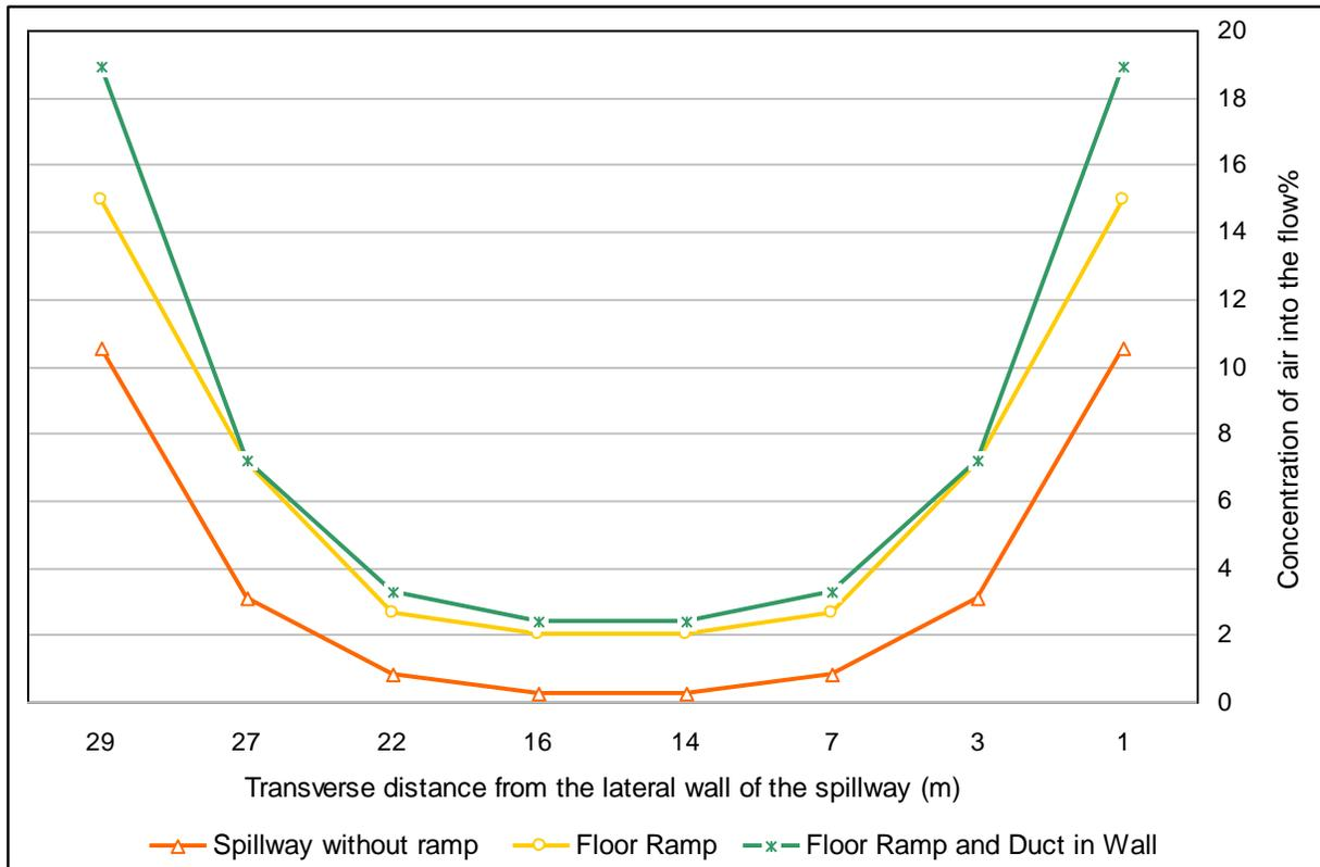
**Figure 6: Changes in the concentration of air into the flow in cross section at a distance of 225 meters from the zero**
