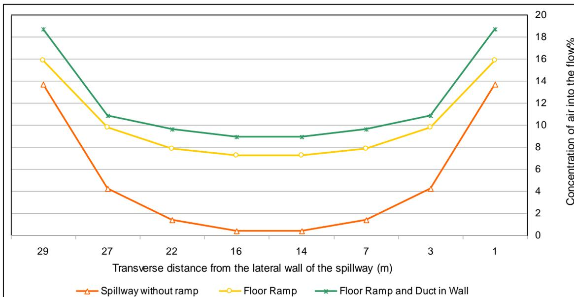
**Figure 5: Changes in the concentration of air into the flow in cross section at a distance of 210 meters from the zero**
