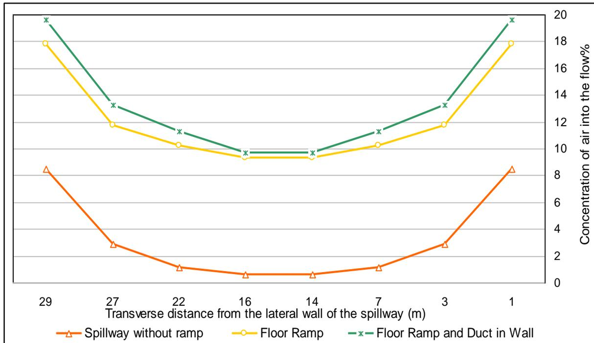
**Figure 7: Changes in the concentration of air into the flow in cross section at a distance of 235 meters from the zero**
