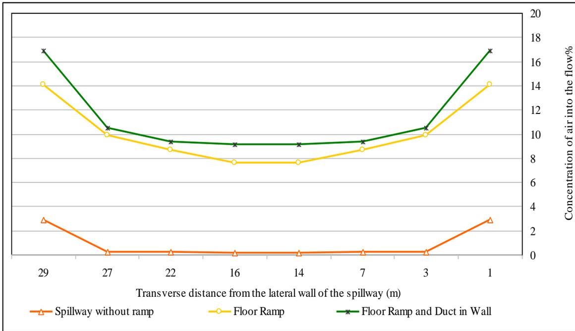
**Figure 4: Changes in the concentration of air into the flow in cross section at a distance of 190 meters from the zero**
