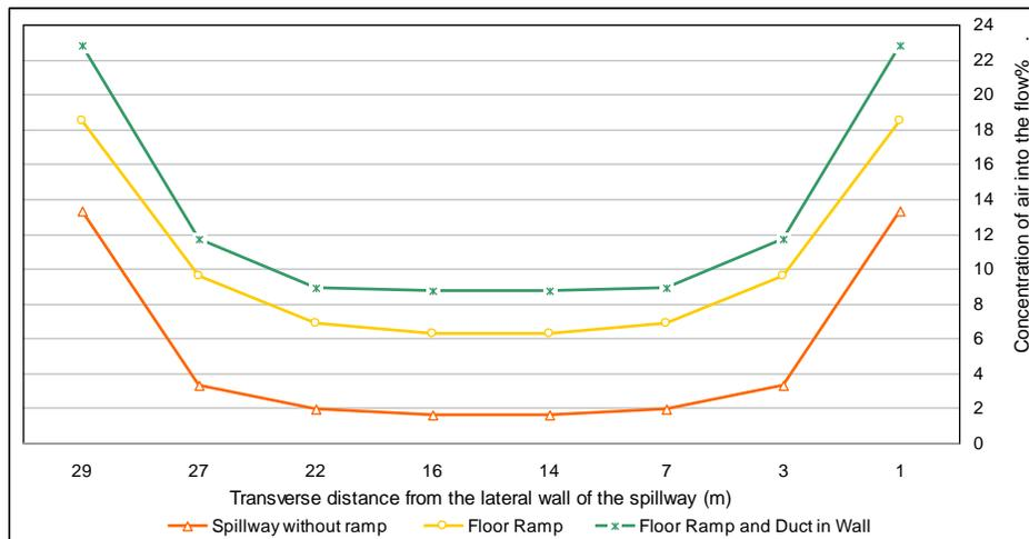
**Figure 9: Changes in the concentration of air into the flow in cross section at a distance of 284 meters from the zero**
