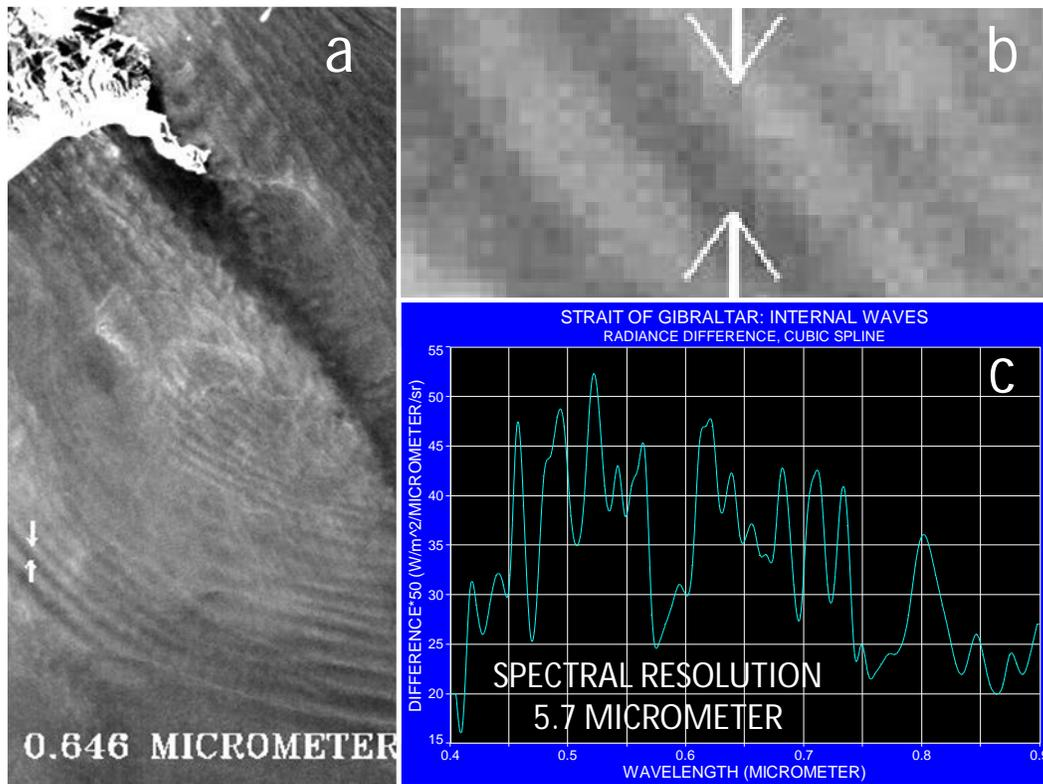
**Figure 1: (a) HICO sub-image showing location where internal waves with a wavelength of about 1000 m were observed at a view angle of 11 degrees to the south/right of the direction of motion of the ISS; (b) enlarged image (a) at 0.646  $\mu\text{m}$  to enhance the presence of internal waves; (c) difference spectrum ( $50 \times$ radiance in  $\text{W m}^{-2} \mu\text{m}^{-1} \text{sr}^{-1}$ ) between bright and darker part of the wave package as indicated by the arrows.**
